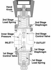
The advantage of a dual stage regulator is its ability to deliver a constant pressure, even with a decrease in inlet pressure. For example, as a
