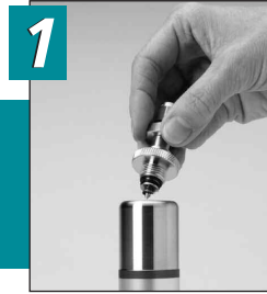
1 Align End Connector into Purifier
