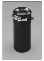
This unit will remove  $O_2$  or water vapor from inert gas carriers such as nitrogen, helium, or argon to less than 1 ppm. Six (6) standard cylinders of 300 cu. ft. are easily treated where the incoming  $O_2$  concentrations are 10 ppm or less.
