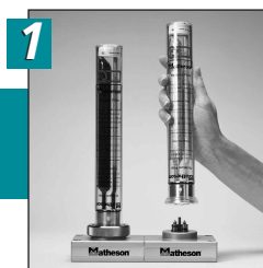
1 Snap cartridge onto base
